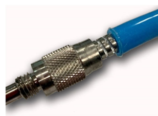
Figure 9 - The sheathing has been pulled away from the end tip, most likely caused by improper handling. Remove this light guide from service
