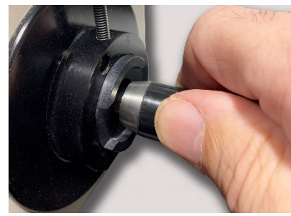
Figure 6 - Always grasp the light guide end fitting by the handle to remove the lightguide from the light source and instrument.
