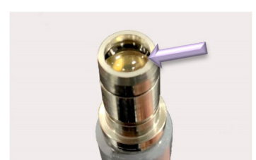
Figure 10 - Medical headlight cable with a lens. Check to make sure the lens is secure, clear, with no cracks.
